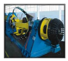
Cable stranding machinery, such as the one pictured, utilize 360 degree rotating arms. Bearings and other components inside the machine are not accessible for condition monitoring.
